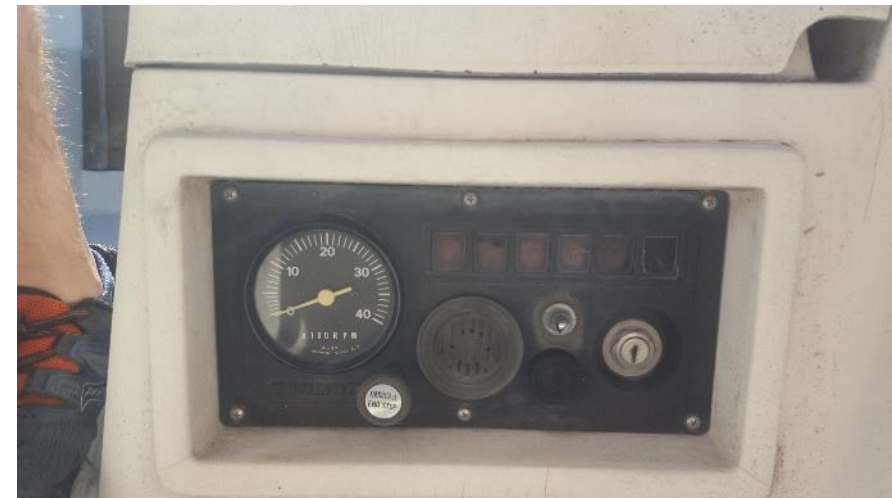
Starting key, kill switch and rpm meter
